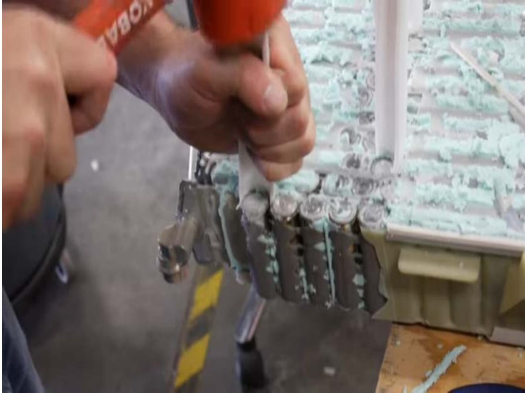
Figure 4. Pack disassembly—thermoplastic materials challenges.
